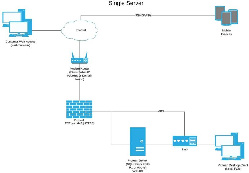
This configuration does not permit desktop client access from outside of the primary physical LAN. If Remote Desktop Services are required, see one of the Multiple Server Configurations
